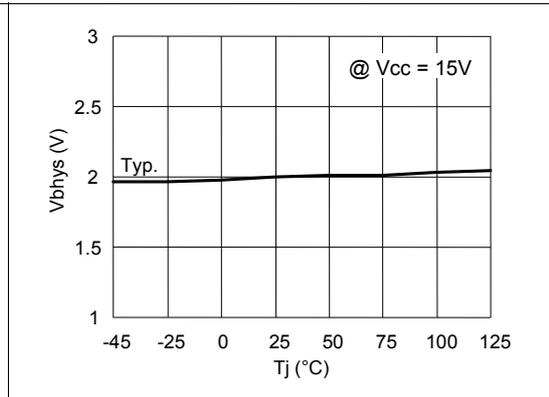
Figure 13. V<sub>CC</sub> UV turn-on threshold vs. temperature
