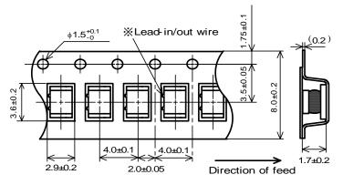
%The packing directions of the chip coil in taping are unified with the in/out positions of the lead wire.
