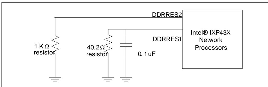
*Note:* Since the OCD calibration function is not enabled, DDRRES2 must be pulled to ground with a 1-KΩ resistor.
