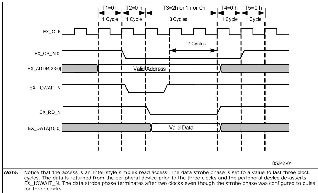
Figure 36. I/O Wait Extended Phase Timing
