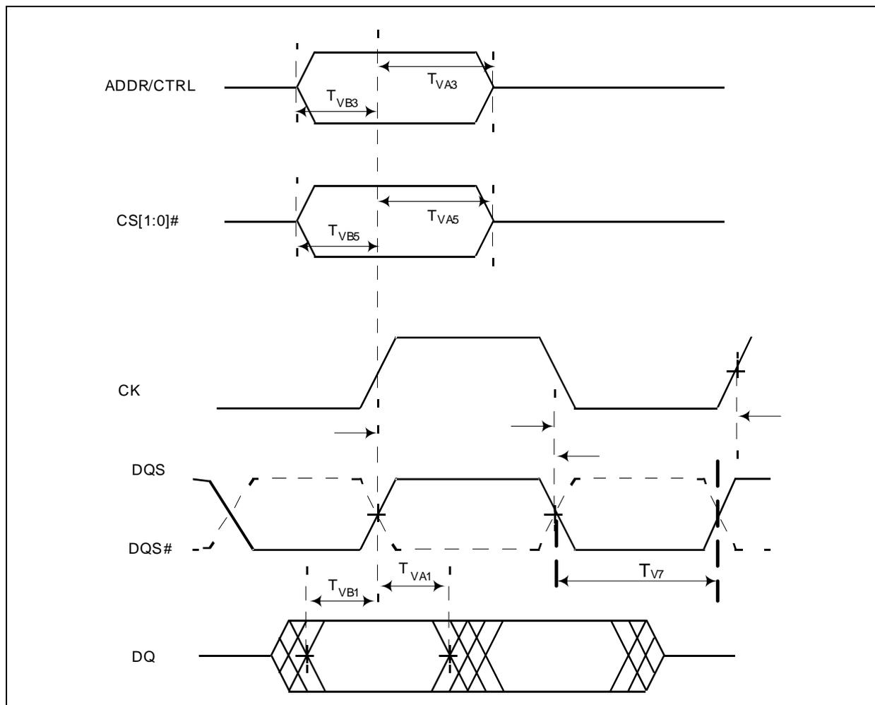
Figure 28. DDR SDRAM Read Timings
