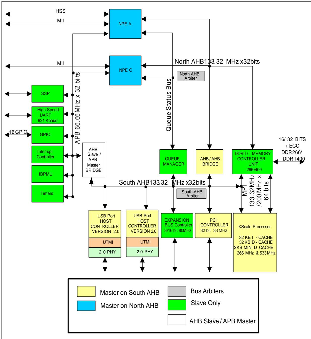
Figure 3. Intel® IXP432 Network Processor Block Diagram
