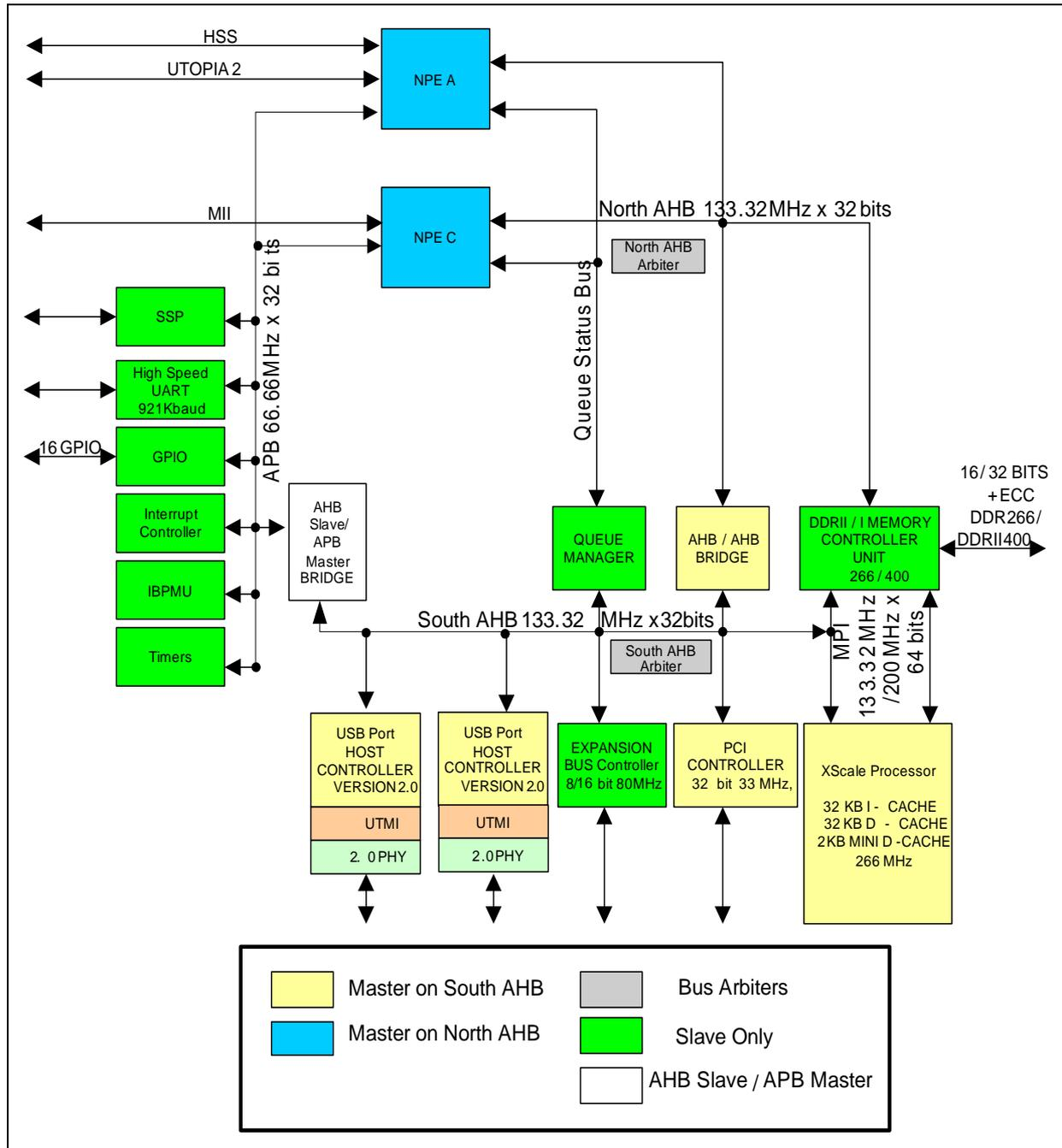
Figure 5. Intel® IXP430 Network Processor Block Diagram
