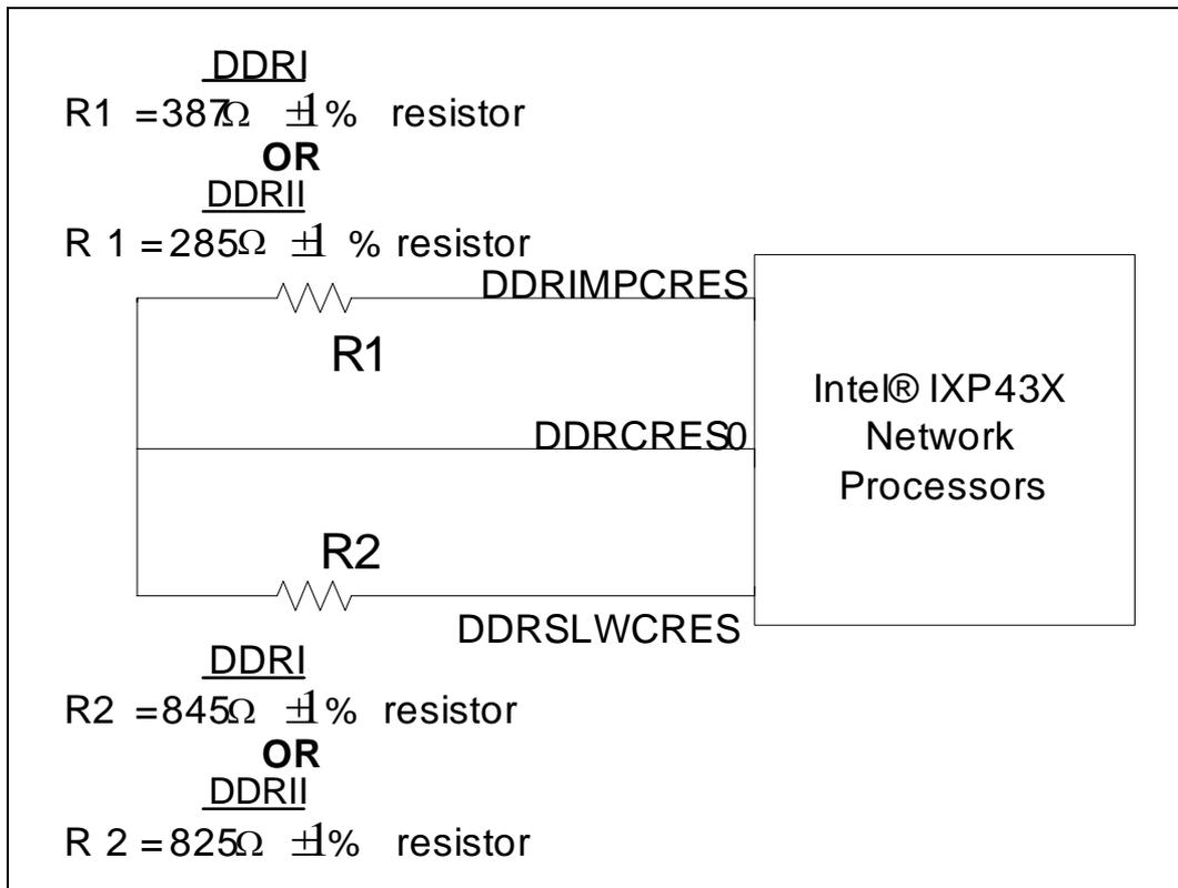
For example, when DDR1 SDRAM is used, DDRIMPCRES is connected with 387Ω and DDRSLWCRES is connected with 845Ω resistor to DDRCRESO.
