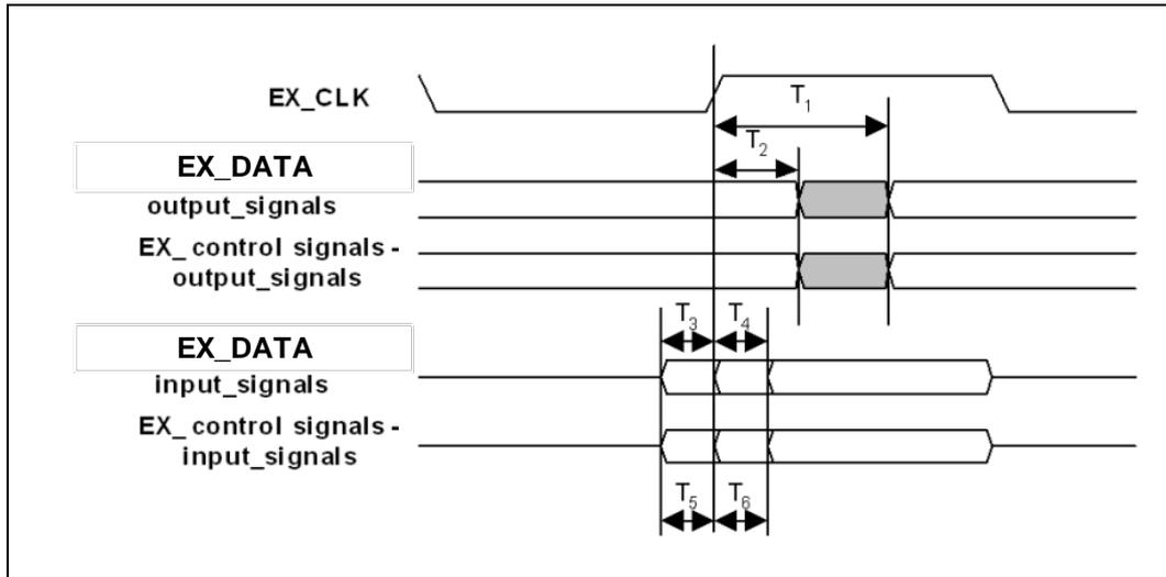
Table 61. Expansion Bus Synchronous Operation Timing Values
