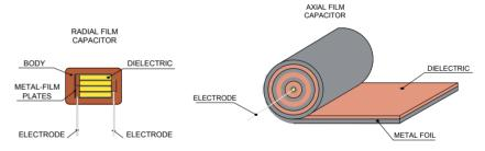
Figure 3.12. Construction of axial and radial film capacitors
