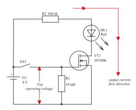
Figure 5.46. An FET as an electronic switch
