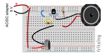
Figure 5.52. Connecting a microphone to FET
