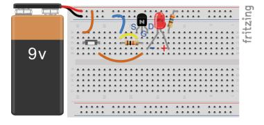
Figure 5.47. Field-effect transistor – electronic switch
