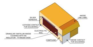
Figure 3.10. Structure of tantalum capacitor
