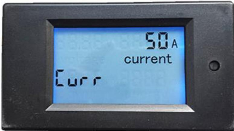
**Step3:** Long press the key to exit the setting state or after no operation within 3 seconds it will store automatically and exit the setting state.
