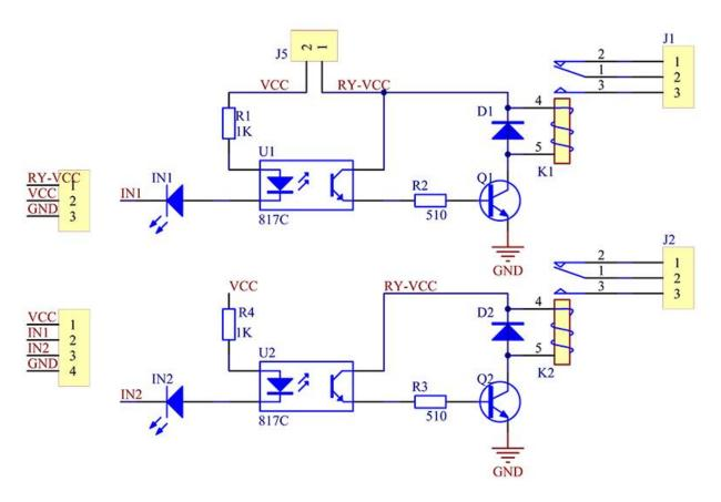
VCC : Connected to positive supply voltage (supply power according to relay voltage)
