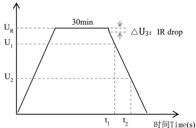
容量计算方式 Capacitance calculation:  $C = I \times \frac{t_2 - t_1}{U_1 - U_2}$
