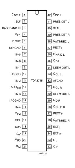
Fig.2 Pin configuration (SDIP42).
